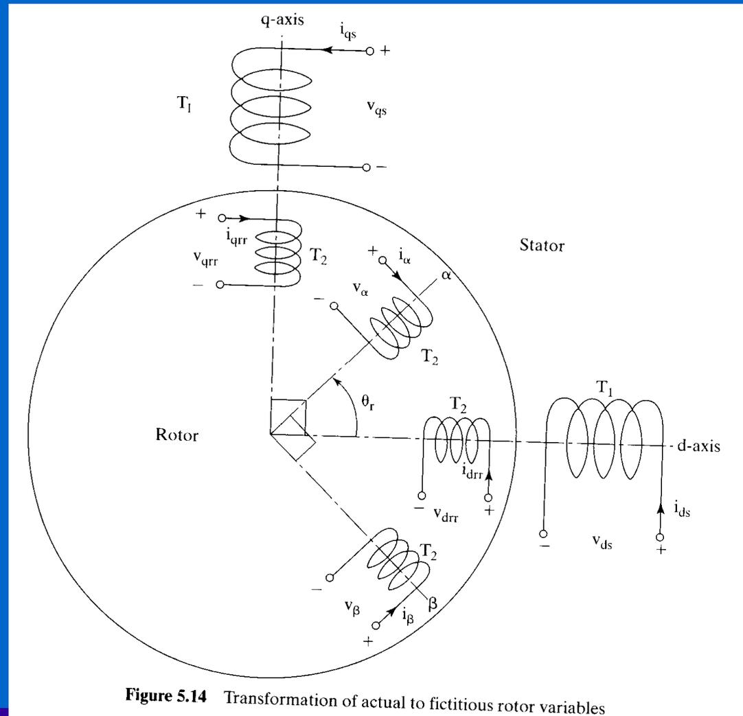
Figure 5.14 Transformation of actual to fictitious rotor variables
