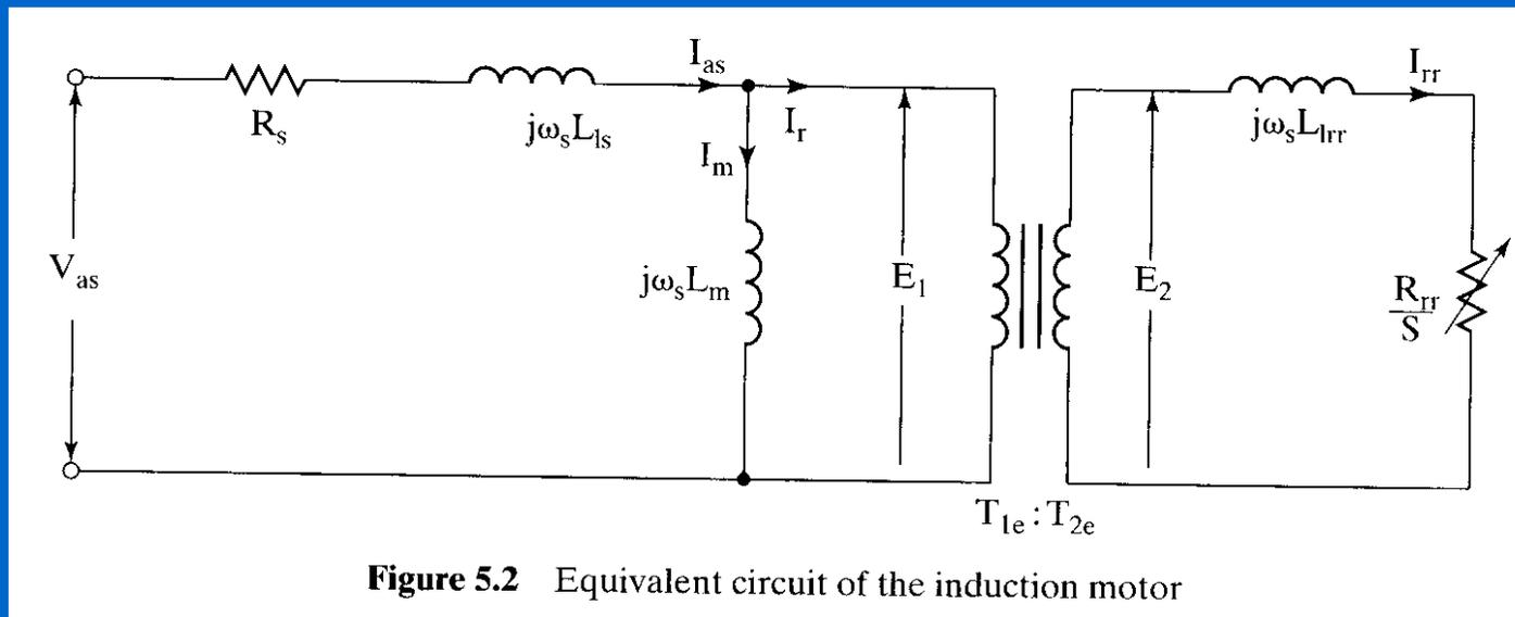
**Figure 5.2** Equivalent circuit of the induction motor
