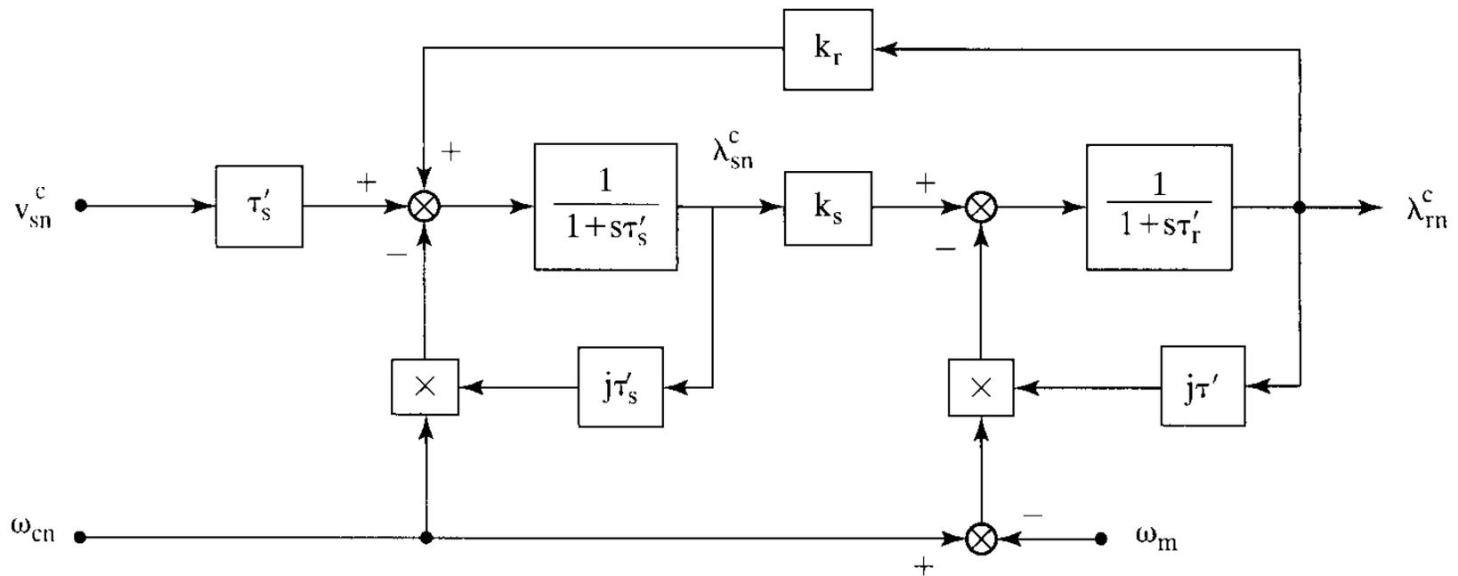
**Figure 5.23** Signal-flow graph of the space-phasor-modeled induction machine
