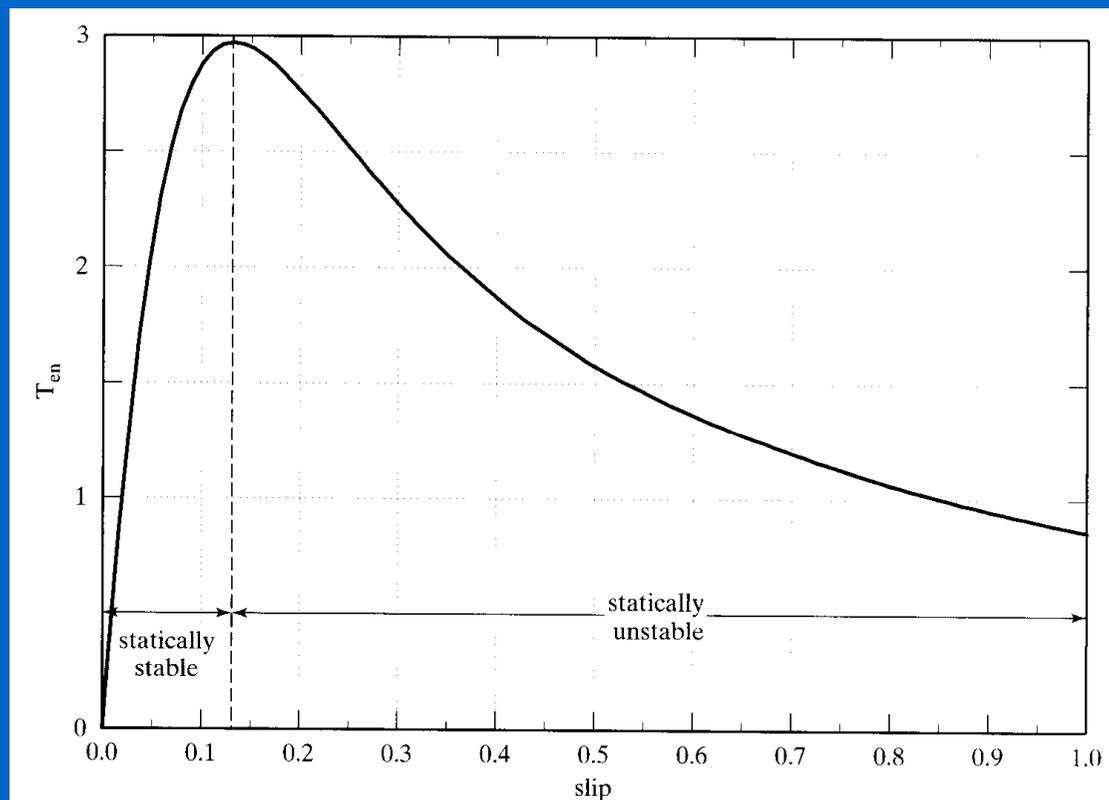
Figure 5.6 (a) Induction motor speed-torque characteristics
