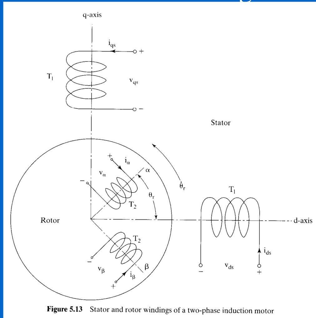
**Figure 5.13** Stator and rotor windings of a two-phase induction motor
