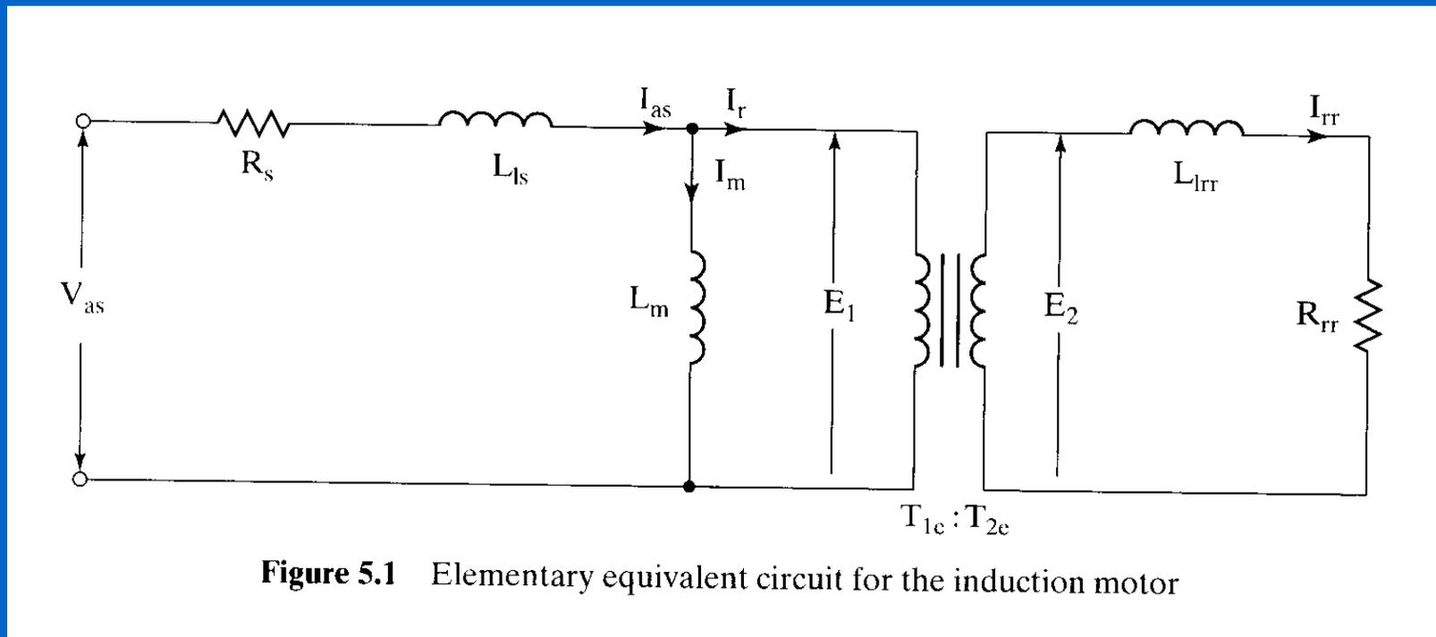
**Figure 5.1** Elementary equivalent circuit for the induction motor
