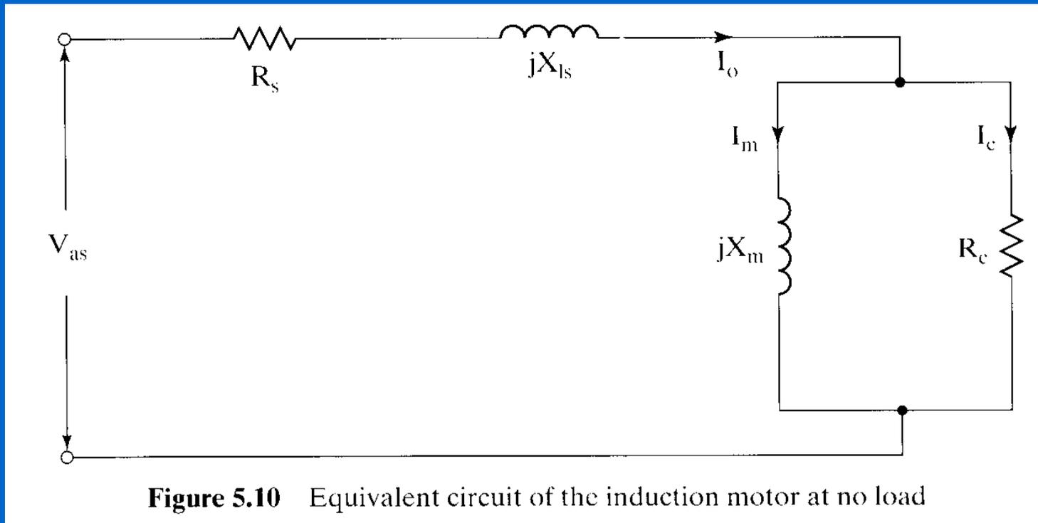
Figure 5.10 Equivalent circuit of the induction motor at no load
