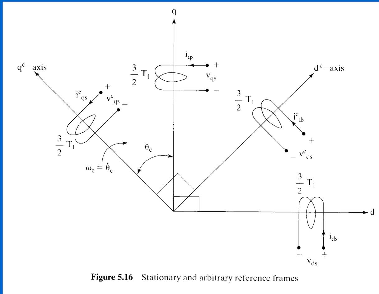
**Figure 5.16** Stationary and arbitrary reference frames
