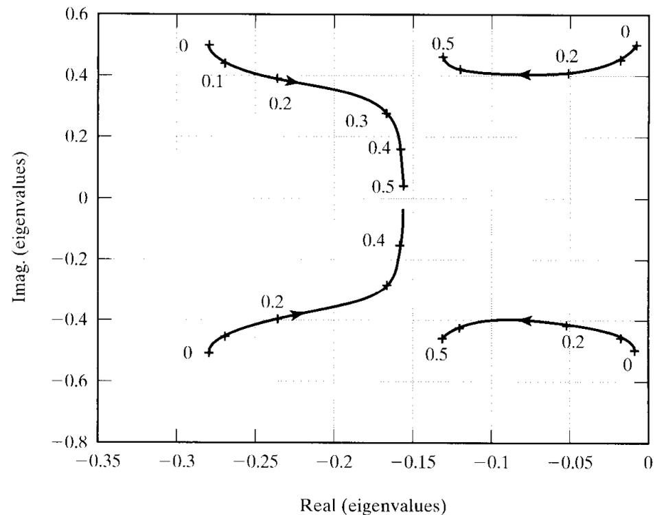
**Figure 5.22** Loci of the eigenvalues in arbitrary reference frames with a velocity of 0.5 p.u. and rotor speed varying from 0 to 0.5 p.u.
